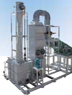
VSC type Venturi scrubber
